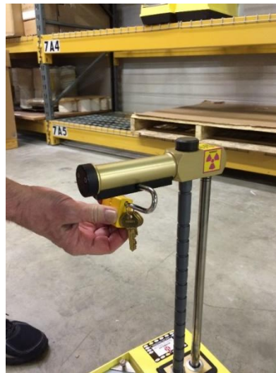
Figure 6 - Installing the Padlock
