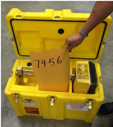
Figure 9 – Installing Documentation Packet
