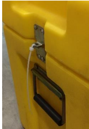
Figure 15 – Zip Tie Attached to Padlock Eyes on the Ends of the Case
