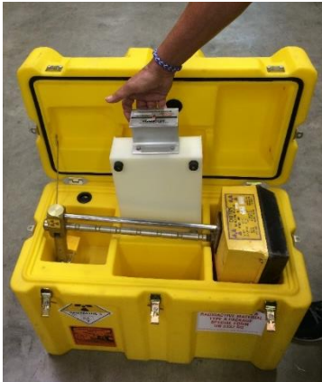
Figure 8 – Installing Reference Standard Block
